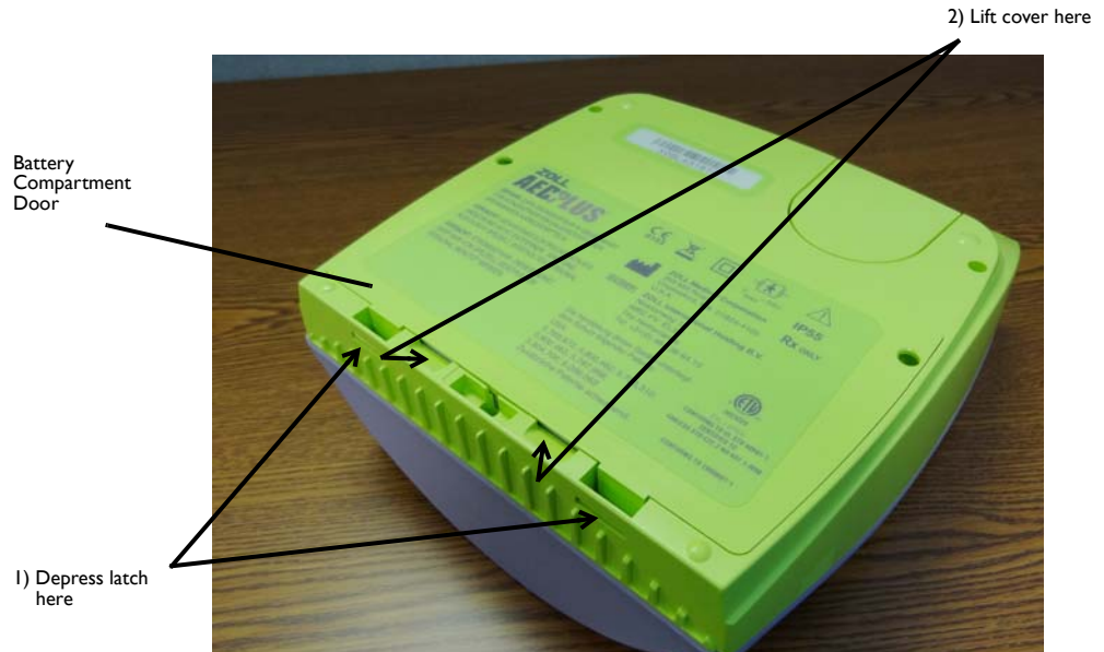
Figure 7: Removing the Battery Compartment Door
