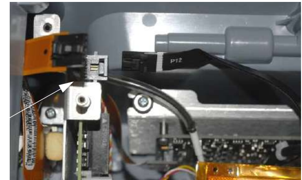
Figure 10.75—Power PCB J12 connection
