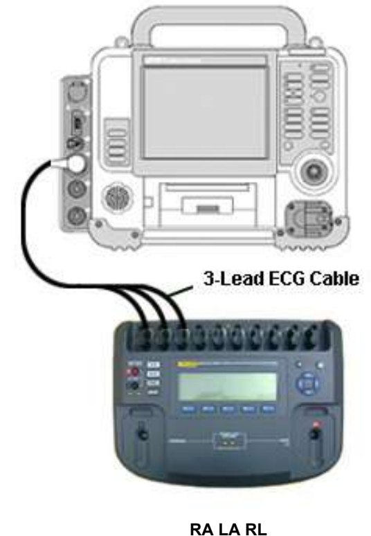
Figure 5.37—ECG 3-wire connection
