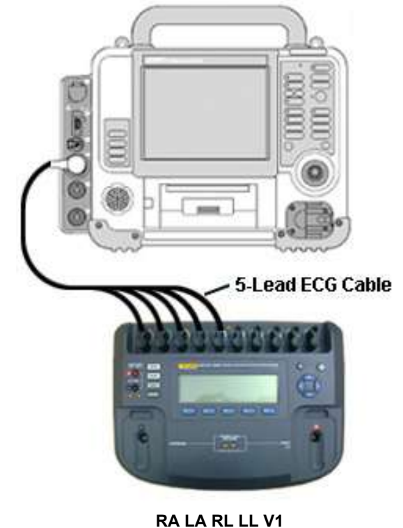
Figure 5.35—ECG 5-wire connection
