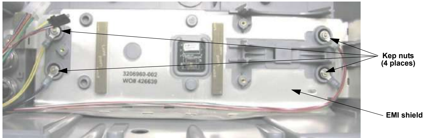
Figure 10.99—EMI shield and battery wire harness nut locations
