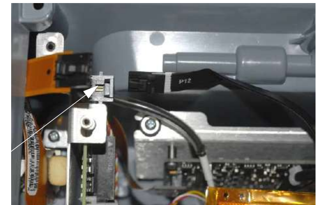
Figure 10.56—Power PCB J12 connection
