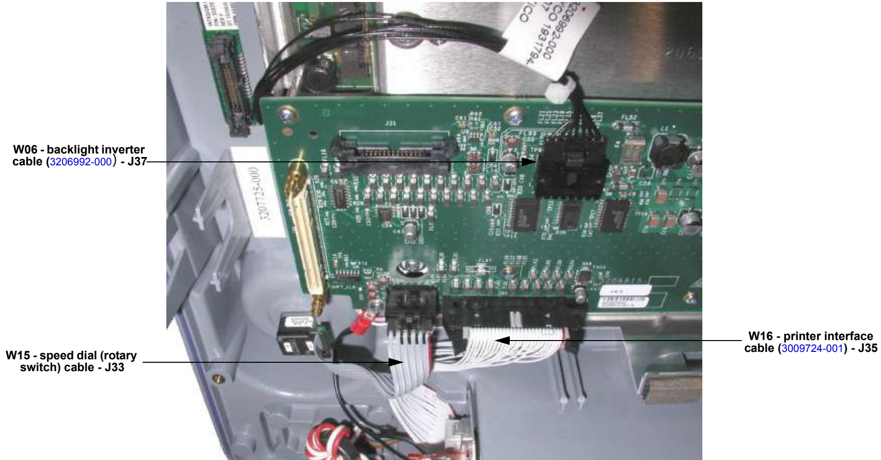
Figure 10.12—Interface PCB cable connection locations - view 2 of 2
