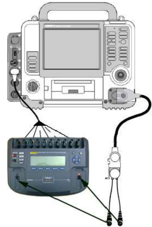
Figure 5.53—Pacer leads-off test setup
