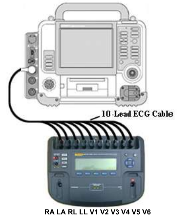
Figure 5.33—ECG lead connections
